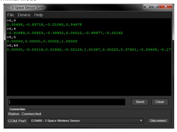
Terminal mode allows you to communicate directly with the sensor without the aid of the graphical interface. For instructions on how to communicate using terminal commands, see the 3-Space Sensor Usage/Protocol section in the 3-Space Sensor User's Manual document.
