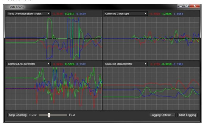
This tool provides various visualizations of the data that can be read from the 3 Space Sensor as well as the ability to log this data to a file.
