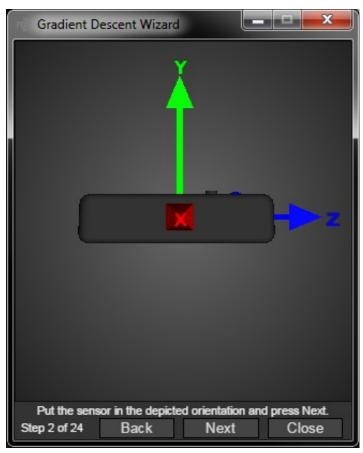
• **Run Gradient Descent Wizard.** This wizard will help you calibrate the compass and accelerometer. First, a screen will appear asking you to select which component sensors you would like to calibrate.
