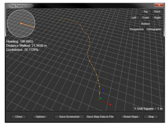
This function tracks movement in space from the sensor's heading and acceleration data. The orientation of the three dimensional representation can be changed with the Top, Back, Left, Front, Right, and Bottom Buttons and the camera can changed to and from Perspective and Orthographic mode. In the top left is a compass showing the heading of the sensor, the distance walked calculated from the sensor readings and the confidence level in the readings.
