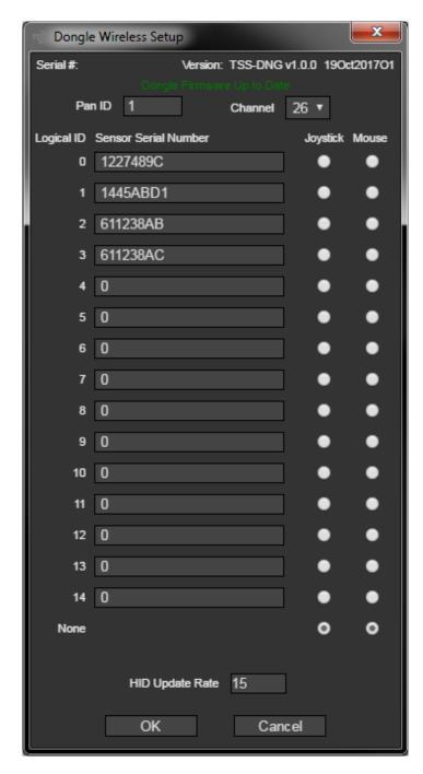
On this screen, enter the serial number of a wireless sensor into the address slot you would like to communicate with it on. You may later select that address in the Sensor Select box on the main window to communicate with that sensor.
