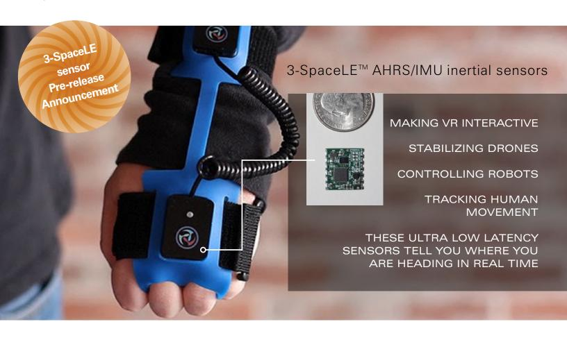
Yost Labs' 3-SpaceLE<sup>TM</sup> sensor is a surface-mountable, miniature, high-precision, high reliability, Attitude and Heading Reference System (AHRS) / Inertial Measurement Unit (IMU), designed to bring aerospace-grade inertial tracking to the consumer electronics market.
